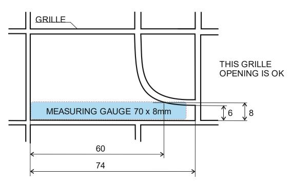
IN THIS EXAMPLE ONE OF THE GRILLE OPENINGS IS MEASURED TO 74mm. BUT THE PERPENDICULAR VALUE (THE HEIGHT) IS LESS THAN 8mm FOR 14mm OF THE DISTANCE. A MEASURING GAUGE WITH A DIMENSION OF 70 X 8mm CAN NOT BE INSERTED.
