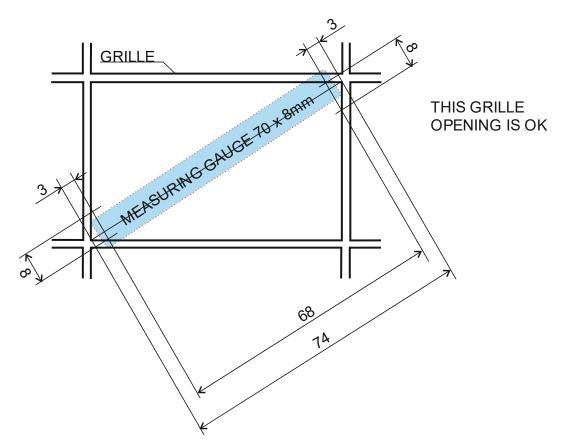
IN THIS EXAMPLE ONE OF THE GRILLE OPENINGS IS MEASURED TO 74mm (DIAGONAL). BUT THE PERPENDICULAR VALUE (THE HEIGHT) IS LESS THAN 8mm FOR 2 x 3mm OF THE DISTANCE. A MEASURING GAUGE WITH A DIMENSION OF 70 X 8mm CAN NOT BE INSERTED.
