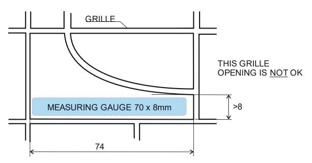
IN THIS EXAMPLE ONE OF THE GRILLE OPENINGS IS MEASURED TO 74mm. THE PERPENDICULAR VALUE (THE HEIGHT) IS MEASURED TO A VALUE EXCEEDING 8mm. A MEASURING GAUGE WITH A DIMENSION OF 70 X 8mm CAN EASILY BE INSERTED.
